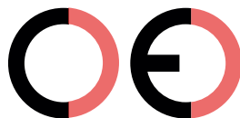
False CE Mark (too far)
